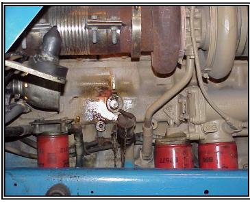
NORTHERN WISCONSIN WEATHER CAUSED FREEZE DAMAGE TO THESE BLOCKS. ABOVE CUMMINS DIESEL AND BELOW GENERAL MOTORS INBOARD ARE REPAIRED IN PLACE WITH MINOR OR NO DISASSEMBLY REQUIRED.
